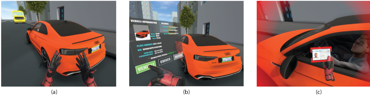
Figure 1: (a) The interface automatically identifies the vehicle’s plate and searches for its information. Color code represents the status of the search. Yellow means that the data is being processed. (b) Once the information is fetched, the interface sends a vibration alert and changes the color code to represent the status of the findings. Green means that the car is clear. The officer can see further information in the arm-mounted display. (c) While checking the driver’s license, the interface identifies a criminal record and sends a red alert. The driver’s record can be seen in the arm-mounted display.
